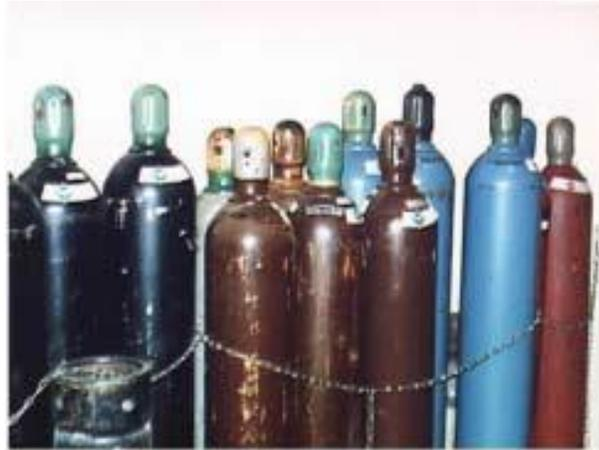
K. Cylinders may be stored outdoors but should be protected from the ground to prevent bottom corrosion. Where extreme temperatures prevail, cylinders should be stored so they are protected from the direct rays of the sun.
